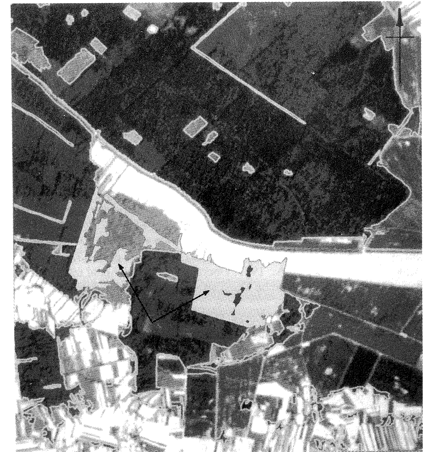
Figure 5: Example of detected land cover change in the period from 1993 to 1997 over an area in updated Land Cover GIS of Slovenia (Gauss-Krüger co-ordinates of the UL corner: X/Y= 5606000/5162000 ) where gray colour (arrow pointed) indicates the extent of the changed wooded land cover to agriculture land use.
